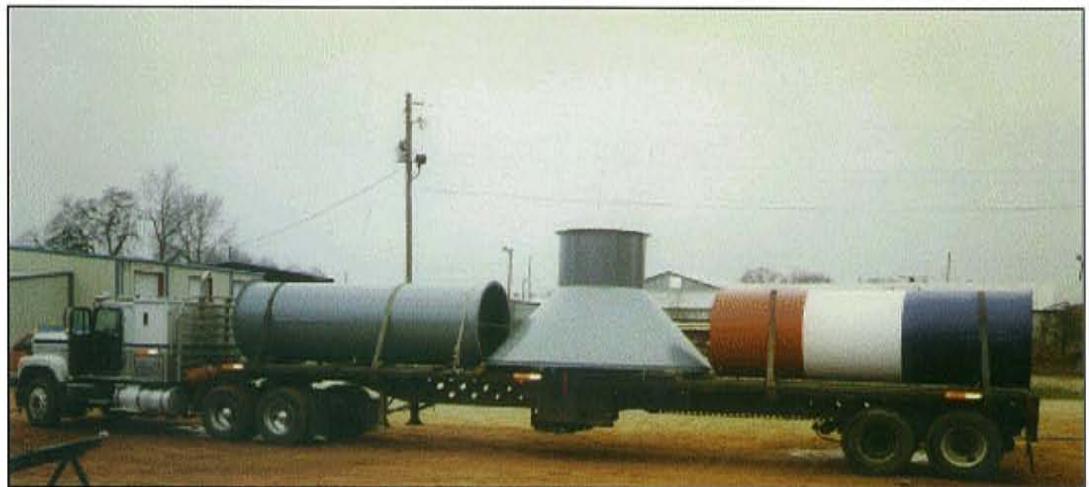
SCRUBBER STACK & CONE BASE
