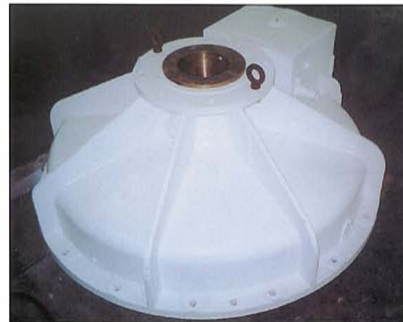
REPAIRED 50" MILL GEAR HOUSING
