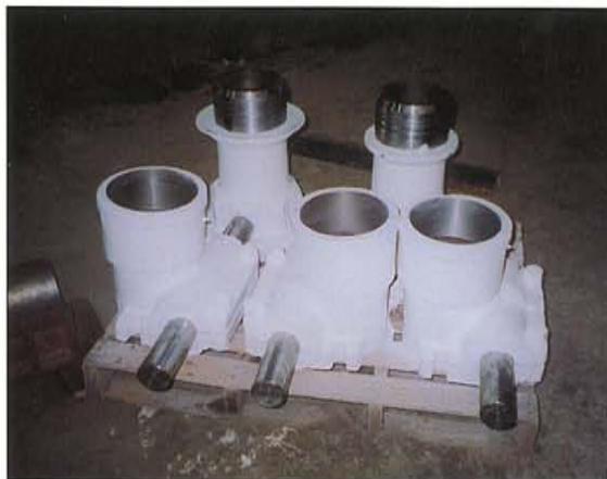
REPAIRED JOURNAL HEADS FOR 73" MILL
