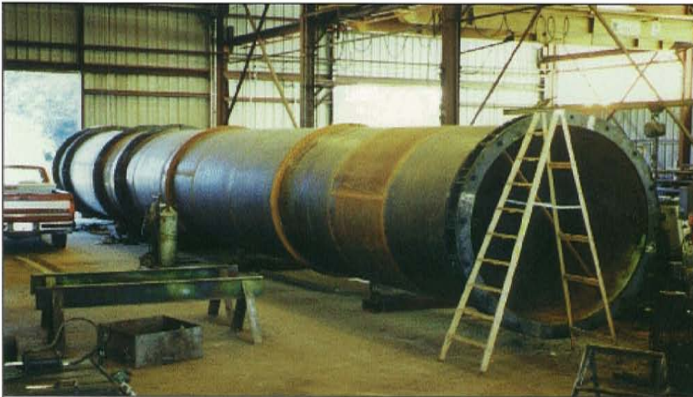
8' X 60' CONVEYOR SUPPORT COLUMN
