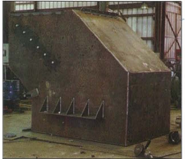
CONVEYOR HEAD CHUTE
