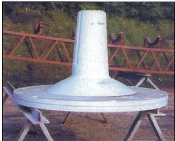
REPAIRED 73" MILL BOTTOM
