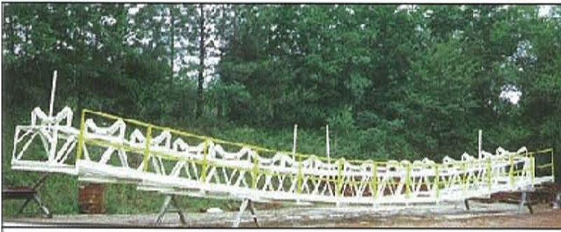
CURVED CONVEYOR SECTION FOR RADIAL STACKER
