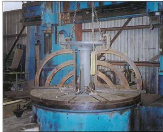
50" MILL BOTTOM CASTING BEING MACHINED
