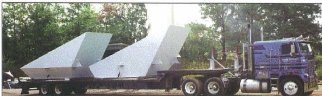
SHIPPING FABRICATED SCREEN CHUTES
